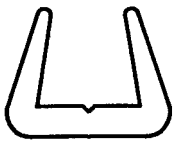
203138-02 Extrusion, plastic panel edging, brown
