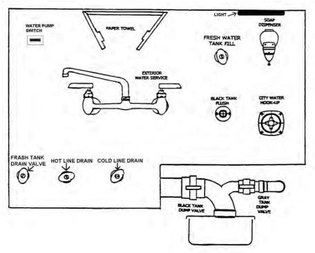
Use a high-pressure hose of at least <sup>1</sup>/<sub>2</sub>" diameter. It should be one that is tasteless, odorless and non-toxic designed for RV use. The city water inlet is a standard garden hose thread. We suggest you carry two lengths of hose. This way you have the ability to reach hookups further away than normal, plus you have a spare hose should one fail or become damaged unexpectedly. Turn the water heater bypass to the normal flow position as described under self-contained.
