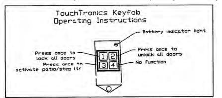
NOTE: When you use the keypad to turn the patio lights ON you must also use the keypad to turn them OFF. The same goes for the switch inside the door ... if you turn the lights on with this switch, you must use the same switch to turn them off. You cannot turn the lights on with the keypad and off with the switch.
