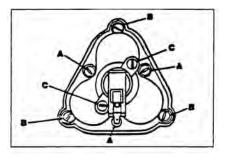
• Screws (C) would be removed to correct a problem in the automatic switch or check valve.
