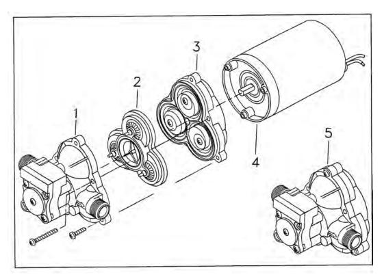
1. Switch/check valve and upper housing kit (replaces all previous switch designs)
