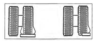
One tire or a portion of one tire is supporting the full load.
