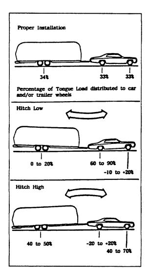
The hitch ball should be level to slightly higher. Readjust leveling bars until this will of condition is correct by increasing or decreasing the length the chain engaged in A frame saddle bracket. Short chain raises hitch ball, longer chain lowers it. A level condition will result in the best balance for towing and steering control as the weight-equalizing hitch distributes the hitch load.
