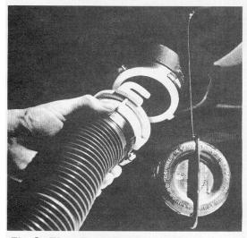
Fig. 5 - Waste Drain Hose Hook-Up
