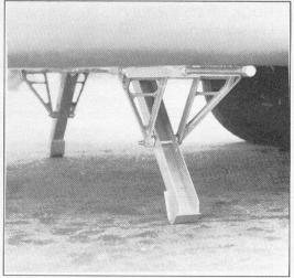
Fig 2 - B.A.L. Stabilizing Jack
