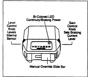
ELECTRONIC CONTROLLERS are inertially activated. The controller senses deceleration and generates an output, which reflects the inertia sensed. When your stationary, the controller does not apply the brakes unless the manual slide bar is activated.
