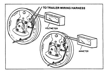
The threshold voltage of a controller is the voltage applied to the brakes when the controller first turns on. The lower the threshold voltage the smoother the brakes will operate. Too high of a threshold voltage (in excess of 2 volts as quite often found in heavy duty controllers) can cause grabby harsh brakes.
