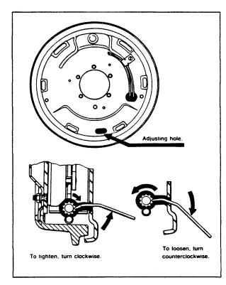
pressure of the linings against the drum makes the wheel very difficult to turn.
