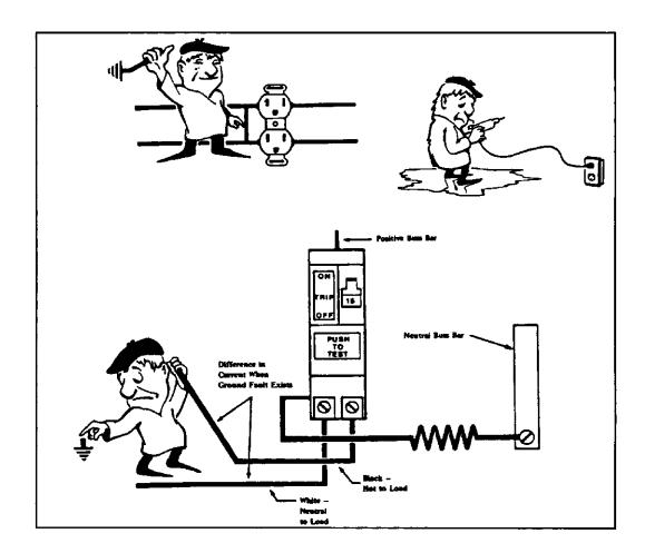
When properly installed, the GFCI circuit breaker provides reliable overload and short circuit protection PLUS protection from Ground Faults that might result from contact with a "HOT" load wire and ground.
