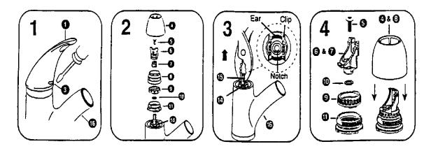
CAUTION: Always turn water OFF before removing existing faucet or disassembling the valve. Open faucet handle to relieve water pressure and ensure that complete water shut-off has been accomplished.
