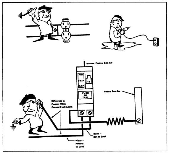
When properly installed, the GFCI circuit breaker provides reliable overload and short circuit protection PLUS protection from Ground Faults that might result from contact with a "HOT" load wire and ground.
