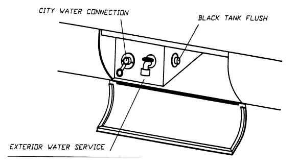
The city water hook-up is found on the lower roadside of the trailer in the utility compartment
