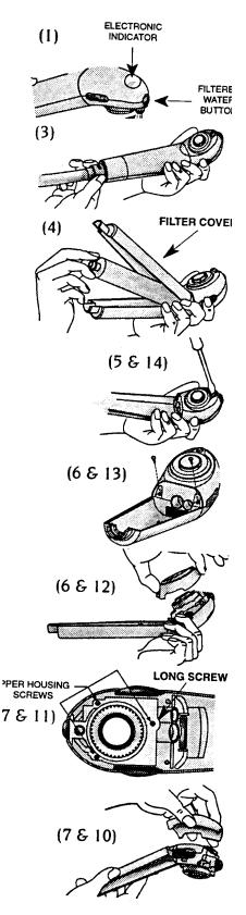
NOTE: When reinstalling screws and filter outlet nut, insert into hole, turn counter clockwise with screwdriver until a click is felt then turn clockwise until snug. DO NOT OVER TIGHTEN!
