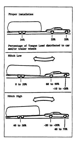
The hitch ball should be level to slightly higher. Readjust leveling bars until this will of condition is correct by increasing or decreasing the length the chain engaged in A frame saddle bracket. Short chain raises hitch ball, longer chain lowers it. A level condition will result in the best balance for towing and steering control as the weight-equalizing hitch distributes the hitch load.
