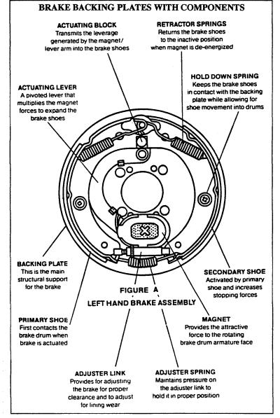
Increasing the current flow to the electromagnet causes the magnet to grip the armature surface of the brake drum more firmly. This results in increasing the pressure against the shoes and brake drums until the desired stop is accomplished.
