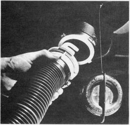
Fig. 5 - Waste Drain Hose Hook-Up
