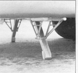
Fig 2 - B.A.L. Stabilizing Jack
