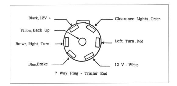
**Note:** The 7 way wire is spliced to the main harness in the area of the 12-volt distribution panel in front of the trailer.
