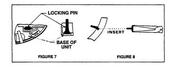
To make the smoke alarm somewhat tamper resistant, a "locking pin" has been provided in the base of the unit. It will help deter a child or other individual from removing the smoke alarm from the bracket. See Figure 7. The following directions can install this.
