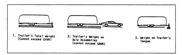
The allowable personal cargo must be distributed in your trailer in such a manner that the Gross Axle Weight Rating is not exceeded.
