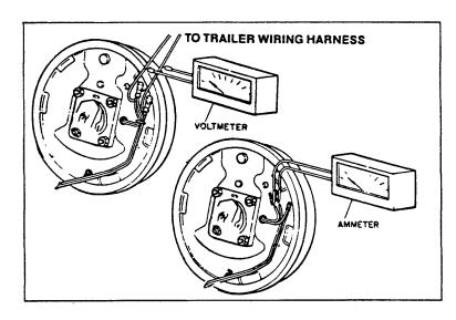
The threshold voltage of a controller is the voltage applied to the brakes when the controller first turns on. The lower the threshold voltage the smoother the brakes will operate. Too high of a threshold voltage (in excess of 2 volts as quite often found in heavy duty controllers) can cause grabby harsh brakes.
