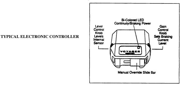
ELECTRONIC CONTROLLERS are inertially activated. The controller senses deceleration and generates an output, which reflects the inertia sensed. When your stationary, the controller does not apply the brakes unless the manual slide bar is activated.
