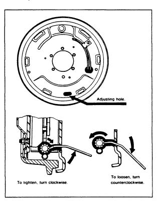
4736 or K-D #295 is recommended.) Adjust the brake shoes out until the pressure of the linings against the drum makes the wheel very difficult to turn.
