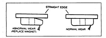
Even if wear is normal as indicated by your straightedge the magnets should be replaced
