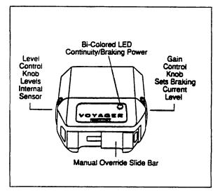
ELECTRONIC CONTROLLERS are inertially activated. The controller senses deceleration and generates an output, which reflects the inertia sensed. When you are stationary, the controller does not apply the brakes unless the manual slide bar is activated.
