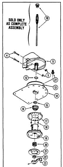
**STEP 7:** Replace directional handle, spring and elevating crank. Make sure setscrew contacts flat on shaft before tightening.
