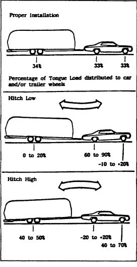
The hitch ball should be level to slightly higher. Readjust leveling bars until this condition is correct by increasing or decreasing the length the chain engaged in "A" frame saddle bracket. Short chain raises hitch ball, longer chain lowers it. A level condition will result in the best balance for towing and steering control as the weight-equalizing hitch distributes the hitch load.
