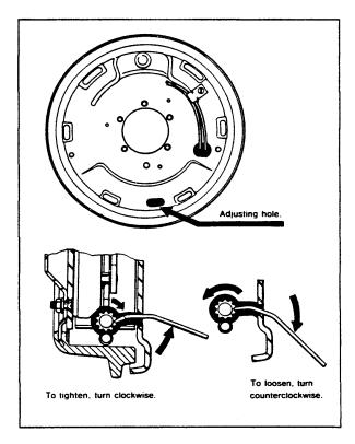
4736 or K-D #295 is recommended.) Adjust the brake shoes out until the pressure of the linings against the drum makes the wheel very difficult to turn.
