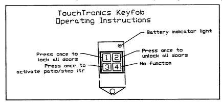
**NOTE:** When you use the keypad to turn the patio lights ON you must also use the keypad to turn them OFF. The same goes for the switch inside the door ... if you turn the lights on with this switch, you must use the same switch to turn them off. You cannot turn the lights on with the keypad and off with the switch.
