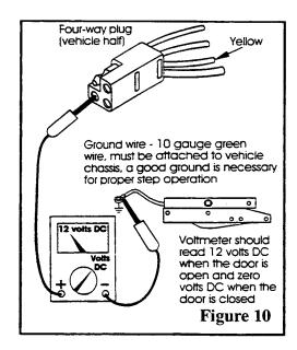
If the reading is zero when the ignition is on, check the terminal connections in the vehicle's fuse/circuit breaker and the condition of the circuit's wiring and terminal connections. NOTE -The step wiring circuit must be independent. No other device (i.e. alarm systems, step well lights, etc.) can be connected to the step wiring circuit. Any device connected to the steps wiring can cause the step to malfunction and will void the warranty.
