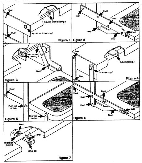
Clean all mud, salt, and road grime from step before lubricating. Lubricate all moving parts (bearings, pivot points, slides, clevis pin, and drive linkage ball) every 30 days with a good quality moisture and heat resistant penetrating grease. Kwik-Lube Spray Grease is specially formulated to lubricate Kwikee Electric Steps and is recommended for lubricating all moving parts. Refer to the figures below for lubrication locations.
