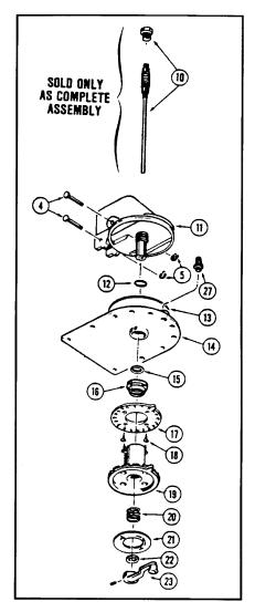
**STEP 6:** Install plastic plug in top of housing, re-engage elevating gear in worm gear, replace pin and retaining ring.
