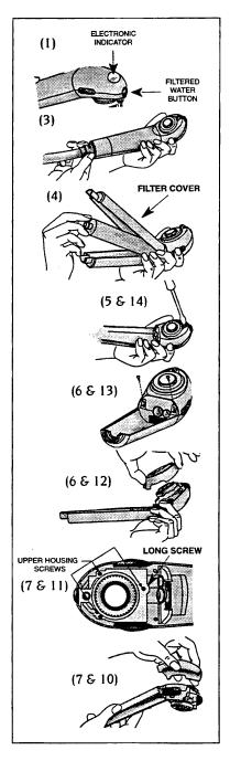
NOTE: When reinstalling screws and filter outlet nut, insert into hole, turn counter clockwise with screwdriver until a click is felt then turn clockwise until snug. DO NOT OVER TIGHTEN!
