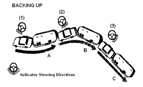
Position (A) start. Turning steering wheel as shown in (1) will put you in trailer position (B). Turning steering wheel shown in position (2) puts you in trailer position (C). Steering position (3) returns front wheels for staright backing.
