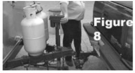
Move the rig ahead about 50 feet and test the trailer brakes, then check the ground for forgotten objects. Regularly check the condition of your tires, air pressure, and the tightness of your lug nuts.
