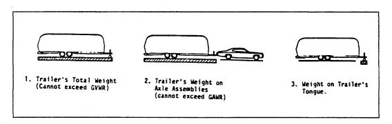
Use a scale, such as a bathroom scale, that has a lower weight limit than your tongue load to check the tongue weight by using the following method (see illustration).
