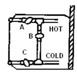
Normal flow position is open valves A and C, close valve B.
