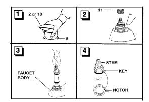
4. To reassemble, reverse the previous steps. Turn the cartridge stem to ON position, so that the hole in the piston lines up with the hole in the outer shell. Plush the cartridge straight down into the body making sure the key on the cartridge fits into the notch in the body. This will correctly position the cartridge. Replace the cartridge nut, start by hand, **DO NOT CROSS THREAD**, and tighten firmly.
