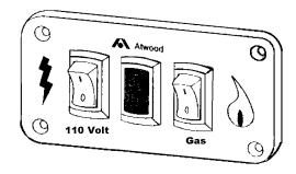
A second switch for the water heater is also located on the panel. This provides power to the heating element. DO NOT use unless you are sure the water heater is full. (Open a faucet and see if there is a full stream of water on the hot side)
