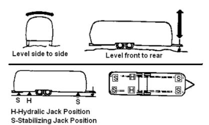
level set on the inside work counter or the trailer hitch "A-Frame". (See Diagram Below) If a correction is necessary then YOU MUST LEVEL FROM SIDE TO SIDE FIRST This can he done easily by backing the trailer up one or more  $2" \times 6"$  boards. (See Diagram) We do not recommend placing tires in a hole for leveling.
