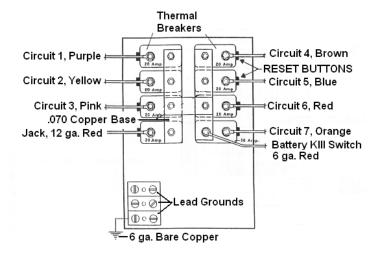
on that circuit. If the breaker continues to trip the system affected should be checked by a qualified service center.
