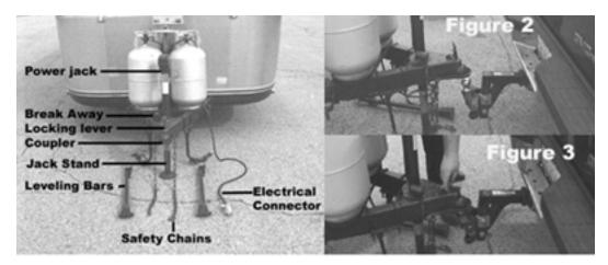
A low hitch ball increases tail wagging tendencies by lowering the nose of the trailer, thus changing the center of support for the trailer and reducing the weight on the four wheels of the tow vehicle. With proper hitch installation and hitching up, the bar should have a noticeable amount of the deflection or bending. A little
