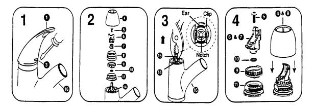
Open faucet handle to relieve water pressure and ensure that complete water shut-off has been accomplished.
