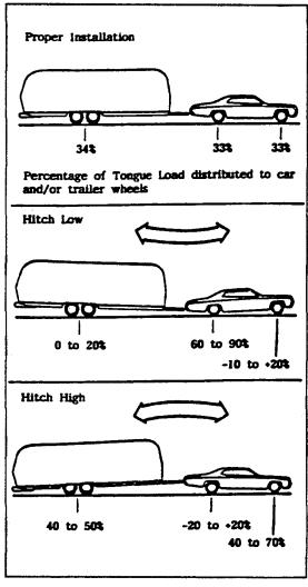
The hitch ball should be level to slightly higher. Readjust leveling bars until this condition is correct by increasing or decreasing the length the chain engaged in "A" frame saddle bracket (Figure 5). Short chain raises hitch ball, longer chain lowers it. A level condition will result in the best balance for towing and steering control as the weight-equalizing hitch distributes the hitch load.
