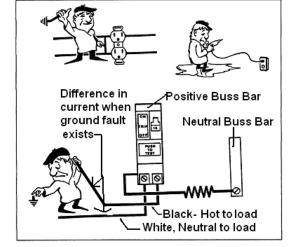
persons can feel as little as 2 milliamperes, a distinct shock may be felt if the need for protection exists. However, the shock should be of such short duration that the effects would be reduced to less than the normally dangerous level. However, persons with acute heart problems or other conditions that can make a person particularly susceptible to electric shock may still be seriously injured.
