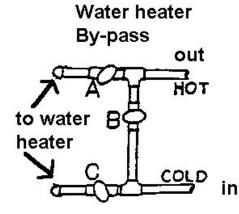
Open valves "A" and "C" and close valve "B" for normal usage. Close Valves "A" and "C", then open valve "B" for winterizing.
