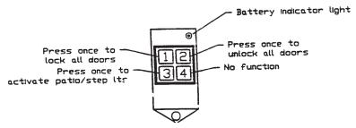
**NOTE:** When you use the keypad to turn the patio lights ON you must also use the keypad to turn them OFF. The same goes for the switch inside the door ... if you turn the lights on with this switch, you must use the same switch to turn them off. You cannot turn the lights on with the keypad and off with the switch.
