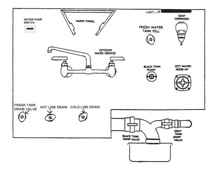
Use a high-pressure hose of at least ½" diameter. It should be one that is tasteless, odorless and non-toxic designed for RV use. The city water inlet is a standard garden hose thread. We suggest you carry two lengths of hose. This way you have the ability to reach hookups further away than normal, plus you have a spare hose should one fail or become damaged unexpectedly.
