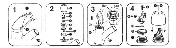
**CAUTION**: Always turn water OFF before removing existing faucet or disassembling the valve. Open faucet handle to relieve water pressure and ensure that complete water shut-off has been accomplished.
