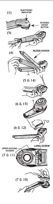
NOTE: When reinstalling screws and filter outlet nut, insert into hole, turn counter clockwise with screwdriver until a click is felt then turn clockwise until snug. DO NOT OVER TIGHTEN!
