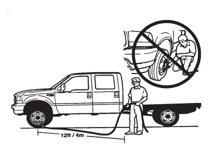
WARNING: An inflated tire and rim can be very dangerous if improperly used, service or maintained. To avoid serious injury, never attempt to re-inflate a tire which has been run flat or seriously under inflated without first removing a tire from the wheel assembly for inspection. Do not attempt to add air to tires or replace tires or wheels without first taking precautions to protect persons and property.
