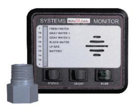
The MicroPulse System makes use of a single solid-state sensor per tank. The MicroPulse sensor measures the static (head) pressure at the bottom of the tank and transmits this information to the MicroPulse System Monitor. Knowing this pressure value, after a one-time calibration has been performed, the MicroPulse System will calculate and accurately display the tank level in 1/8 increment.
