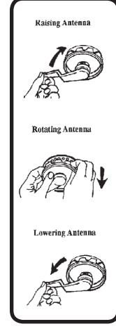
Turn elevating crank in the "Down" direction until resistance is noted. Antenna is now locked in travel position.
