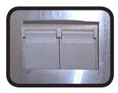
Located on the side of your trailer is a gray electrical inlet with dual covers. Lifting these covers reveals the receptacles to connect cable TV and telephone lines to your trailer.
