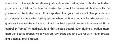
Proper synchronization of tow vehicle to trailer braking can only be accomplished by road testing. Brake "lockup, grabbiness, or harshness" is quite often lack of synchronization between the tow vehicle and the trailer being towed, too high of a threshold voltage (over 2 volts), or under adjusted brakes.
