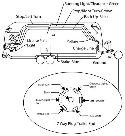
Wire Routing, 7-Way Plug, Battery Charge Line, Distribution Panel
