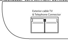
The Cable TV/Telephone inlets are located on the roadside sidesheet on all rear bed models.
