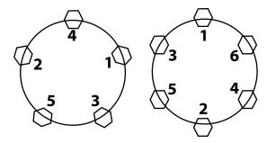
NOTE: Use a torque wrench to tighten lug nuts. Tightening by hand or with an impact wrench is not recommended.
