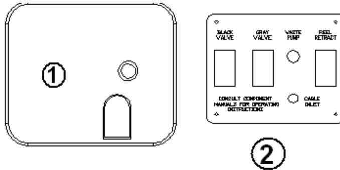
1. 382083W Hatch, sidewall switches w/cable inlet hole, White
