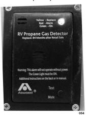
This alarm has a seven year life; see end-of-life notification in LPG detector manual. Please read entire detector manual before operating unit.
