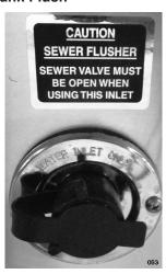
The trailer has a water hose connector specifcally for flushing the Black Water Tank. To use, hook up a hose and turn on full force. Within the tank, a spray head with a multiple holed head will spray the interior surface of the tank. The vacuum breaker and check valve will be located inside the trailer above the exterior connection. In most models, this will place them under the lavatory.
