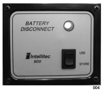
When the switch is turned to USE (on) and the trailer is plugged into a 110-volt shoreline, the 12-volt distribution panel will receive power from the converter and the batteries will be charged through the converter charging system.
