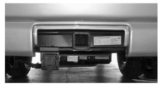
Kneel down behind the rear bumper. There are two slide latches on the rear cover located on the lower backside of the cover. Both will need to be slid to the inside to be unlatched properly as shown below.
