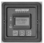
Magnum Inverter/Charger is a DC to AC inverter and a 50-amp multi-stage battery charger. It has a remote control module mounted in the roadside rear roof locker.
