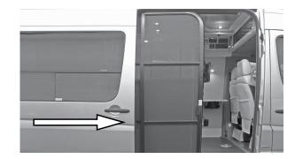
Do not shut the exterior door when the screen door is closed. The screen door must be open before you shut the exterior side door.
