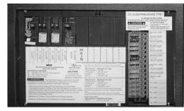
All Interstate models have the Power Center installed at the base of the bed. Open the decorative door for access to 12-volt fuses and 110-volt breakers.
