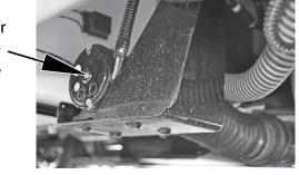
After long periods of non-use, a stuck impeller can be easily broken loose with a screwdriver inserted in the motor shaft slot. Remove the rubber boot, turn the shaft clockwise, and replace the rubber boot.
