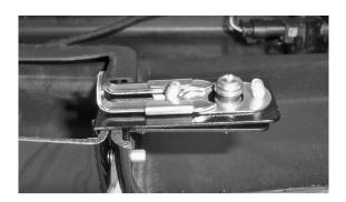
2. Push outer latch past the pin on both sides to release as shown below.
