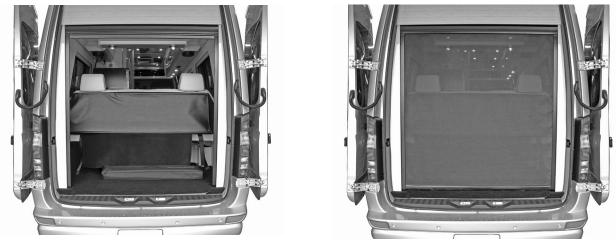
To lower the power screen, press the down button on the remote control. The screen will stop when it reaches the lowest position. To raise the power screen, press the up button on the remote control. You can stop the screen at any point by pressing the opposite direction button on the remote control.
