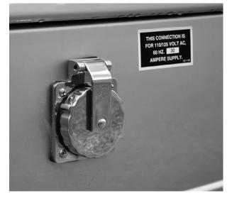
The Power Cord hookup is located on the side of the motorhome. The cord may be stored in the rear exterior compartment. The power cord is plugged into the motorhome receptacle and the City Power Service.
