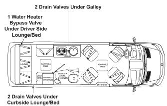
The fresh water system has five fresh water line low point drain valves. There are two under the galley accessed by removing the drawer and two under the curbside lounge or bed accessed by removing the cup holders. The cup holders lift up and out of the armrest, and one water heater bypass valve located under the driver side lounge or bed.
