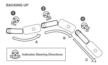
Start in position (A) start. Turning steering wheel as shown in (1). will put you in trailer position (B). Turning steering wheel show in position (2) puts you in trailer position (C). Steering position (3) returns front wheels to straight backing.
