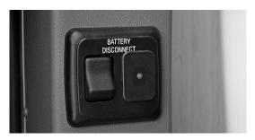
The manual disconnect switch, located inside the rear lounge door on the rear lounge model and on the front of the roadside twin bed on the twin bed model, is used to turn off power from the battery to the 12-volt distribution panel.
