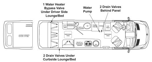
The fresh water system has five fresh water line low point drain valves. There are two beside the fridge in front of the storage area accessed by removing the panel and two under the curbside lounge or bed accessed by removing the cup holders. The cup holders lift up and out of the armrest, and one water heater bypass valve located under the driver side lounge or bed.
