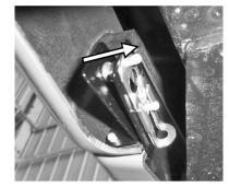
3. Pull straight down to remove cover. Once removed you can store this in one of the rear storage compartments. Reverse these instructions to reinstall.
