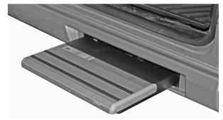
The curbside sliding door has a sliding step with auto retract, step out warning buzzer, and a lock extended switch located just inside the sliding door on the forward shower wall. Please read, understand, and instruct passengers of the following operational and safety information pertaining to the step.
