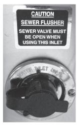
The trailer has a water hose connector specifically for flushing the Black Water Tank. To use, hook up a hose and turn on full force. Within the tank, a spray head with a multiple holed head will spray the interior surface of the tank. The vacuum breaker and check valve will be located inside the trailer above the exterior connection. In most models, this will place them under the lavatory.
