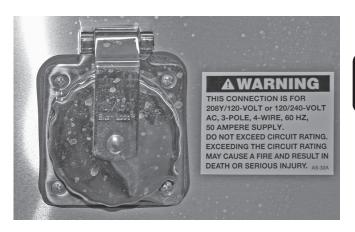
The Power Cord hookup is located on the side of the trailer. The cord may be stored in the rear exterior compartment. The power cord is plugged into the trailer receptacle and the City Power Service.
