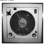
The optional high-volume roof vent system is designed to quickly exhaust stale, hot air and draw in fresh air. It is great to use when the outside temperature does not call for air conditioning, but heat has built up in your coach.
