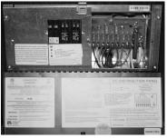
All International models have the converter installed on the front lower portion of the pantry, at the base of the bed, or at the front of the L-lounge. Open the decorative door for access to 12-volt fuses and 110volt breakers.
