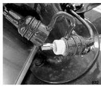
Should an electrical failure occur, remove the power head by loosening the two Allen setscrews. The jack post may now be operated manually by inserting the emergency handle into the coupling on top of the post.
