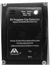
This alarm has a seven year life; see end-of-life notification in LPG detector manual. Please read the entire detector manual before operating the unit.
