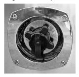
Use a tasteless, odorless, non-toxic, high-pressure hose of at least 1/2-in. diameter designed for RV use. The city water inlet is a standard garden hose thread. We suggest you carry two lengths of hose in order to reach hookups farther away than normal, as well as to have a spare.
