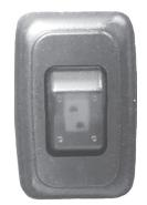
The fan increases the cooling efficiency of the refrigerator; therefore Airstream recommends leaving the switch on whenever possible. Please note that turning the fan off during hot, humid weather conditions may substantially affect the cooling capacity of the refrigerator.
