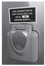
The Power Cord hookup is located on the side of the trailer. The cord may be stored in the rear exterior compartment. The power cord is plugged into the trailer receptacle and the City Power Service.
