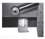
Under the trailer are galvanized steel boxes that are a few inches lower than the trailer frame. These boxes are insulated exterior tank pans and they support the freshwater and holding tanks. Petcocks open with a 1/4 turn; line drain valves are open when the widest part of the oval valve handle aligns with the water line.
