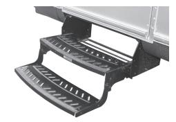
To operate the step, lift up on the front of the step and pull straight out until step locks into place. Some units will be equipped with a double step. After extending the step, the second portion folds out. To store the step, fold it back into position, lift the front slightly and push the step back into its storage area.
