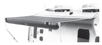
LED light strips have been installed with your awning providing accent lighting. The LED lights are operated by a dimmer switch located on the side of the galley to the right of the entry door.
