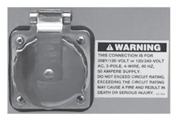
The Power Cord hookup is located on the side of the trailer. The cord may be stored in the rear bumper compartment. The power cord is plugged into the trailer receptacle and the City Power Service.
