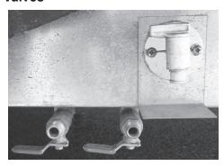
Under the trailer are galvanized steel boxes that are a few inches lower than the trailer frame. These boxes are insulated exterior tank pans and they support the freshwater and holding tanks. Petcocks open with a 1/4 turn; line drain valves are open when the widest part of the oval valve handle aligns with the water line.
