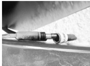
Should an electrical failure occur, first check to see if the fuse has blown. If the fuse is not blown and the jack still will not operate you can manually operate the jack by placing the manual override handle into the alignment tube and engaging the drive pin. Rotating the handle counterclockwise to raise or clockwise to lower the trailer. If the fuse is blown, replace the fuse with the same type and check to see if the jack is now operable.
