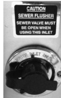
The trailer has a water hose connector specifically for flushing the Black Water Tank. To use, hook up a garden hose and turn it on. Within the tank, a head with multiple holes will spray the interior surface of the tank. Once the tank is about half full, turn the garden hose off and flush the water from the tank using the dump valve. The valve should be closed for the first couple of minutes, and then opened to let the water out in a rush. Repeat as needed.
