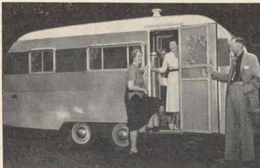
This is an absolutely "go anywhere" trailer. The tandem wheels on such a little light weight job give it towability you never dreamed of. Takes the gallop out of uneven roads. Very little hitch weight, No overload springs of any kind needed.
