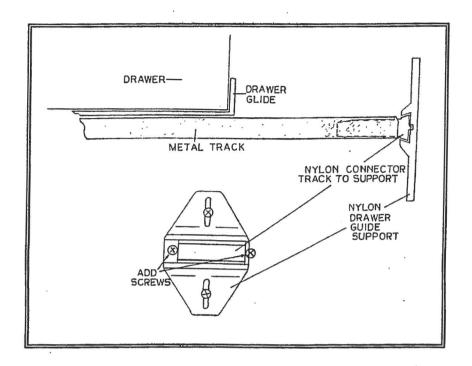
\* This style drawer glide was used in many different locations. If you have other drawers with the nylon connector sliding out of the drawer guide support, adding the screws as shown will correct the problem. Note: The connector is not necessarily centered. Slide the drawer closed and make sure the drawer is square to the cabinet face. Carefully slide the drawer out and secure the connector in the position that it assumed when the drawer face was square.
