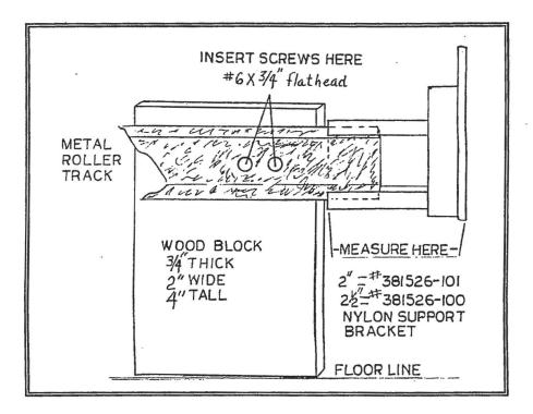
If the nylon support bracket is broken and replacement is required, there are two different designs. To obtain the correct parts measure the support bracket as shown in the illustration and reference that part number corresponding to that measurement. When ordered by part number you will receive a pair — right and left.
