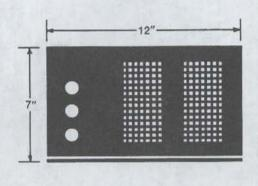
Leave 3" clearance on sides and top or install in compartment of not less than 1.5 cu-ft. Do not obstruct ventilating openings, overheating may result.
