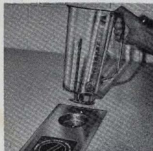
1. Place blender in position on Power Unit. Turn clockwise to lock securely.
