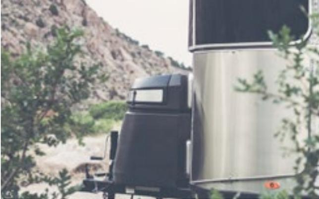
In order to keep the inside of the Basecamp safe, LP gas has to be stored in specific locations where it can't vent into the trailer. That's why we designed our own patented LP storage compartment and cover on the front of the Basecamp. It's made of a special thermal plastic that surrounds the entire LP system, and it's hollow, so if there is a gas leak, it will vent out the bottom and into the fresh air.
