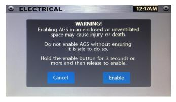
Once enabled, AGS will remain enabled until the Sprinter Ignition is cycled or the generator is manually operated. After the vehicle is started, the AGS will be disabled. You can then return to the cabin to manually re-enable the system. It will then remain active until the vehicle is turned off. Any cycling, on or off, of the vehicle ignition will disable the AGS functionality.
