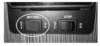
The battery disconnect switch located on the multiplex panel at the entry door is used to separate the 12-volt distribution panel from the converter charging system. When connected to an external AC power source, the 12-volt distribution panel will receive power from the converter and the touring coach will function normally. The batteries will be charged through the converter charging system regardless of if the battery disconnect switch is in the ON/OFF position.
