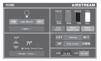
The "Home" screen of the Multiplex Systems main control panel displays the fluid levels of the Black Water, Grey Water, Fresh Water, and the LP gas tanks. The panel also shows the voltage status of the main (chassis) and the auxiliary (house) batteries.
