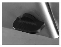
3. Pull straight down to remove cover. Once removed you can store this in one of the rear storage compartments. Reverse these instructions to reinstall.
