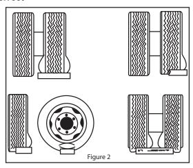
INCORRECT methods are shown in Figure 2: One tire, a portion of one tire, or portions of two tires are supporting the full load.
