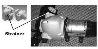
To clean the strainer screen: with the clear plastic at the top, press on the sides of the strainer releasing the tabs holding the clear plastic top in place, hold the sides in, and pull straight up on the clear plastic top to remove the screen assembly. Rinse all debris from the screen. Replace the screen assembly by aligning the screen in the seating groves and pressing gently down until tabs catch and hold the clear plastic top in place.
