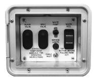
Remove the high pressure waste hose by opening the hose reel compartment door and momentarily pressing the "release" switch. Once released the hose can be manually pulled out. Secure the hose at the disposal facility inlet using the threaded or rubber adaptor and open the drip proof valve on the end of the hose.
