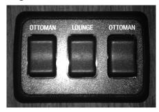
The side ottomans and rear lounge can be converted into a sleeping area by first pulling out the aluminum extension, lowering the pillow extenders, and removing the headrests. Press and hold the switch located under the passenger side overhead storage locker until the lounge flattens completely. This same switch will be located on the driver's side in the Grand Tour model. Lower the powered ottomans on each side of the coach to complete setup.
