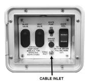
The touring coach is also pre-wired for a portable satellite antenna. The exterior inlet is located on the side of the touring coach and is labeled for your convenience. The interior pre-wire, consisting of a two-pin power/ground connector and a coax cable pigtail, is located in the front roof locker under the Blu-Ray.
