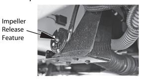
After long periods of non-use, a stuck impeller can be easily broken loose with a screwdriver inserted in the motor shaft slot. Remove the rubber boot, turn the shaft clockwise, and replace the rubber boot.
