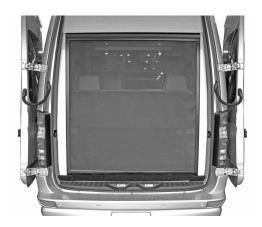
To lower the rear power screen, press the down button on the multiplex control panel once. To stop the power screen in the position that you want, press the button again or allow the screen to stop automatically when it reaches its set limit. To raise the power screen back up press the up button on the multiplex control panel.
