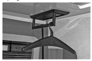
A collapsing clothes rod is located below the rear overhead, behind the rear lounge/bed.
