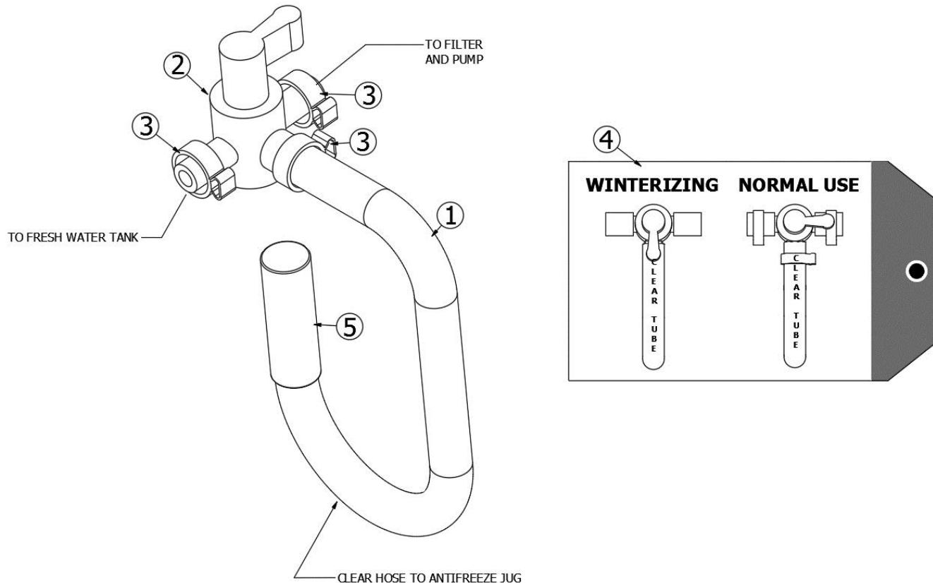
1. 601240-01      Tubing 1/2 I.D. X 3/32 Wall Thick
