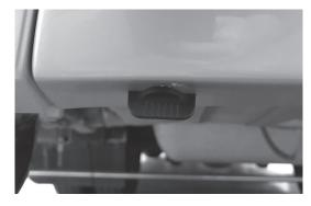
2. Rotate each wing nut 1/4 turn, pull down and remove.
