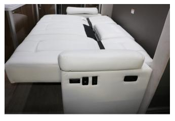
The power sofa is also used as the base support for the murphy bed. Clear the surrounding area of any obstructions before you begin. Remove the dinette table and store in the drawer at the base of the sofa. Make sure the sofa is in its normal upright position and not reclined. Press and hold the right arrow switch located on the side of the sofa. Lower the sofa fully until it stops and release the switch. To return the sofa to its upright position press and hold the left arrow switch.
