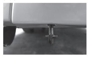
Pull straight down to remove the cover. Once removed you can store this in one of the utility compartments. Reverse these instructions to reinstall.
