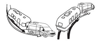
During practice, observe that the tracks made by the trailer wheels are distinctly different from those made by the tow vehicle. Studying this will make it easier for you to correct mistakes. Consider truck- or trailer-type fender or door grip rear view mirrors for maximum visibility. In most states, the law requires them.
