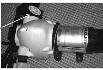
To clean the strainer screen: With the clear plastic at the top, press on the sides of the strainer releasing the tabs holding the clear plastic top in place, hold the sides in, and pull straight up on the clear plastic top to remove the screen assembly. Rinse all debris from the screen. Replace the screen assembly by aligning the screen in the seating groves and pressing gently down until tabs catch and hold the clear plastic top in place.
