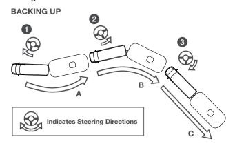
Start in position (A) start. Turning steering wheel as shown in (1). will put you in trailer position (B). Turning steering wheel show in position (2) puts you in trailer position (C). Steering position (3) returns front wheels to straight backing.
