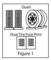
The CORRECT methods are shown in Figure 1. Dual tires are supporting the full load. Please note that the blocks are wider than the tread and longer than the tire's footprint. This provides maximum support to the tires and ensures that the load is evenly distributed throughout the tire's footprint area.
