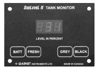
The display is the only system component that is accessed by the user. The display shown above is located in the entry cabinet behind the passengers seat. All user input to the display is done using the four buttons along the bottom of the display.
