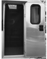
The screen door is secured to the threshold of the main door and can be operated independently by sliding and latching it via a magnet catch. This innovated door takes a fresh approach to maximizing fresh air and your view while offering a smooth and steady screen operation.
