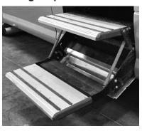
The curbside door has a folding double step with auto retract, step out warning buzzer, and a lock extended switch located just inside the door. Please read, understand, and instruct passengers of the following operational and safety information pertaining to the step.
