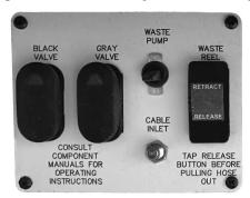
Remove the high pressure waste hose by opening the hose reel compartment door and momentarily pressing the "release" switch. Once released the hose can be manually pulled out. Secure the hose at the disposal facility inlet using the threaded or rubber adaptor and open the drip proof valve on the end of the hose.
