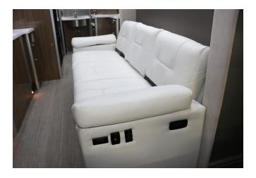
The sofa has power adjustment controls, located on the outside of each armrest, used to recline each end of the sofa. Also located on each armrest is a set of USB ports for plugging in your electronic devices.
