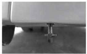
3. Pull straight down to remove the cover. Once removed you can store this in one of the utility compartments. Reverse these instructions to reinstall.
