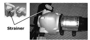
To clean the strainer screen: With the clear plastic at the top, press on the sides of the strainer releasing the tabs holding the clear plastic top in place, hold the sides in, and pull straight up on the clear plastic top to remove the screen assembly. Rinse all debris from the screen. Replace the screen assembly by aligning the screen in the seating groves and pressing gently down until the tabs catch and hold the clear plastic top in place.
