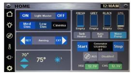
The "Home" screen of the Multiplex Systems main control panel displays the fluid levels of the Black Water, Grey Water, Fresh Water tanks, and the LP gas tanks. The panel also shows the voltage status of the main (chassis) and the auxiliary (house) batteries.
