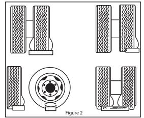
INCORRECT methods are shown in Figure 2: One tire, a portion of one tire, or portions of two tires are supporting the full load.
