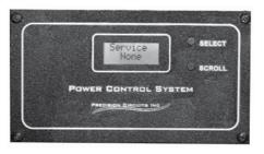
The display panel requires little user interaction and is provided to help the user understand power management. The display monitors the total AC current of the touring coach and prevents circuit breaker tripping by momentarily shedding loads. As additional appliances are turned on the system will begin to shed loads. As appliances are turned off, and a minimum of two minutes has expired, the system will automatically restore power to each of the shed loads.
