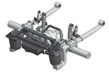
The touring coach is equipped with a rear axle air suspension. The Mercedes-Benz Sprinter Van is extremely suited for this air suspension system.
