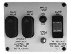
1. Remove the high pressure waste hose by opening the hose reel compartment door and momentarily pressing the "release" switch. Once released, the hose can be manually pulled out. Secure the hose at the disposal facility inlet using the threaded or rubber adaptor and open the drip proof valve on the end of the hose.
