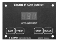
The display is the only system component that is accessed by the user. The display shown above is located in the entry cabinet behind the passengers seat. All user input to the display is done using the buttons along the bottom of the display.
