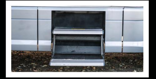
The powered step automatically extends and retracts when the door opens.
