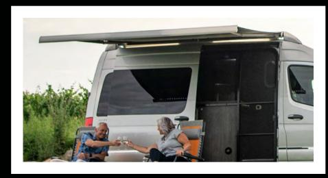
The powered awning extends and retracts at the push of a button.
