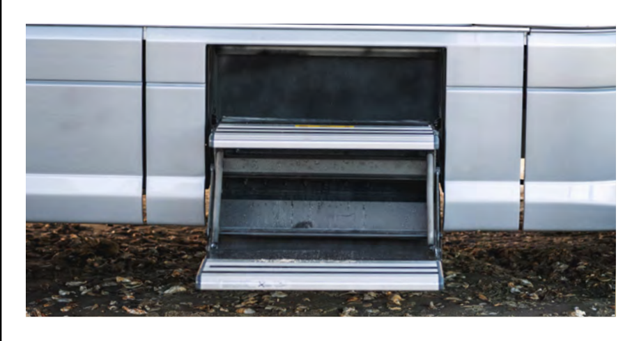
1 The powered step automatically extends and retracts when the door opens.
