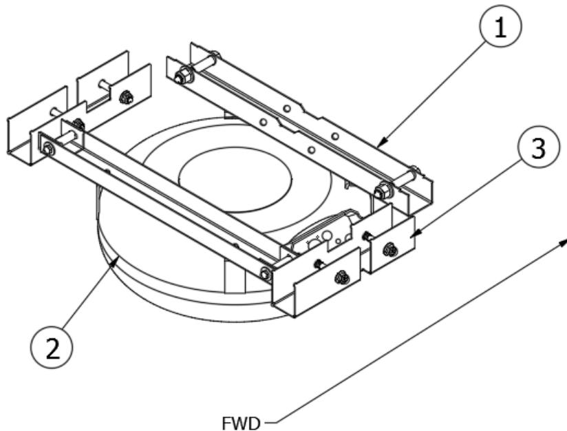
113172      Install - Lp Tank, Toroidal
