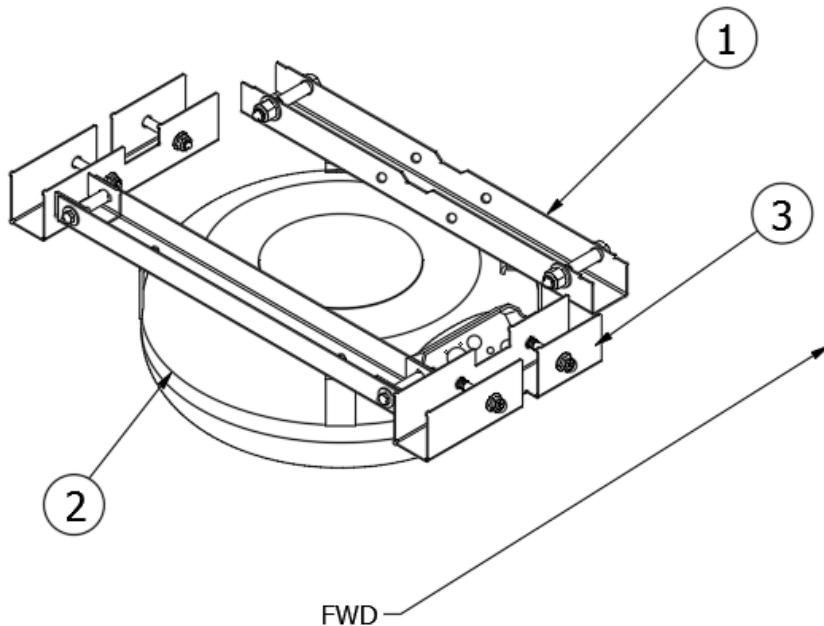
113172      Install - Lp Tank, Toroidal
