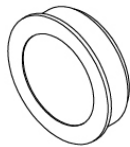
COMPOST GROMMET VENT SCREEN 113910A SCALE 1:1
