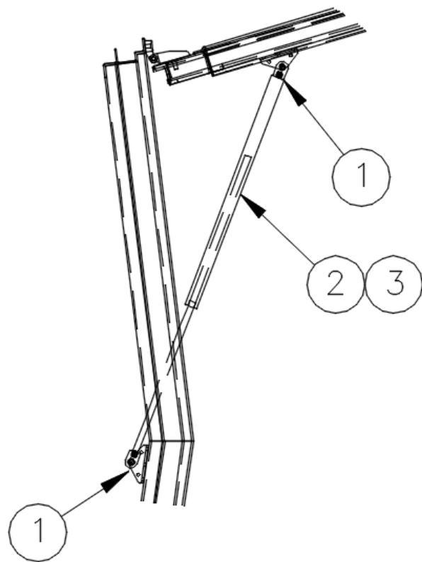
111935                  Install, Struts, Hatch Door (not for order/see parts below)
