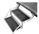
To operate the step, lift up on the front of the step and pull straight out until step locks into place. After extending step, the second portion folds out. To store the step, fold it back into position, lift the front slightly, and push the step back into its storage area.
