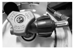
The LPG tanks are equipped with fill valve connections *RV Type I Acme*. The large, green, nylon swivel nut is a right-hand thread and is designed for hand operation only.
