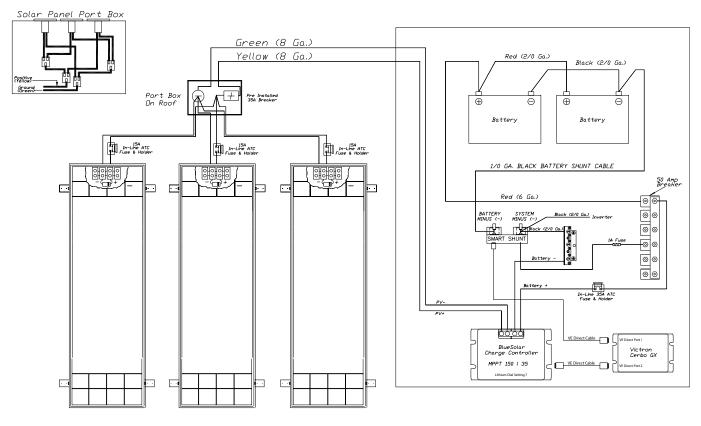
\*Solar Grounds to Battery via Ground Buss bar.
