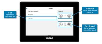
The controls for the roof vent have been incorporated into the Multiplex System. The vent lid can be operated by pressing the Open/Close buttons in the climate control menu on the Multiplex control panel. Pressing the fan button once will turn the vent fan on low. Press the button a second and third time for medium or high. Pressing the button a forth time will turn off the fan.
