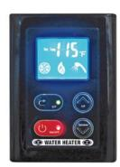
The trailer is equipped with a continuous water heater featuring freeze protection, and direct spark ignition. The tankless water heater monitors inlet water temperature and flow, and output water temperature and flow. The water heater is operated by the control panel located on the wall above the galley sink. Turn on the power and press the temperature selection arrow to see the current setting. Set the desired temperature using the up or down arrows.
