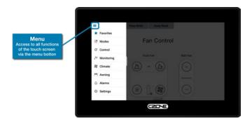
Pressing the "Menu" button, located at the top left corner of the touch screen, accesses the CZone® sub menus. This Menu will provide the user controls and information ranging from lights and temperature controls to alarms and notifications.
