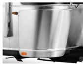
Stainless steel rock guards protect the front end from road debris. You can clean behind the rock guards by swinging them forward on their hinges. They are locked in place with two acorn-style nuts, removable with a 7/16" wrench.
