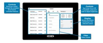
The Controls Menu provides a list of everything controlled by the CZone<sup>®</sup> system. Scroll UP or DOWN on the left side of the screen to view the list. Tap the screen when the feature you want to control is displayed. The right side of the screen will change to display the control options associated with that feature. Some basic feature information will also be displayed.
