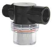
Locate the strainer housing (on the water line leading to the water pump inlet). Remove the transparent bowl (turn counterclockwise), and carefully pull out the strainer/screen. Clean and rinse with water (use a household detergent if necessary). Reinstall the strainer and bowl, being careful not to damage the seal. The bowl collects sediment and should be positioned under the housing as depicted above. Check for leaks prior to resuming normal operation.
