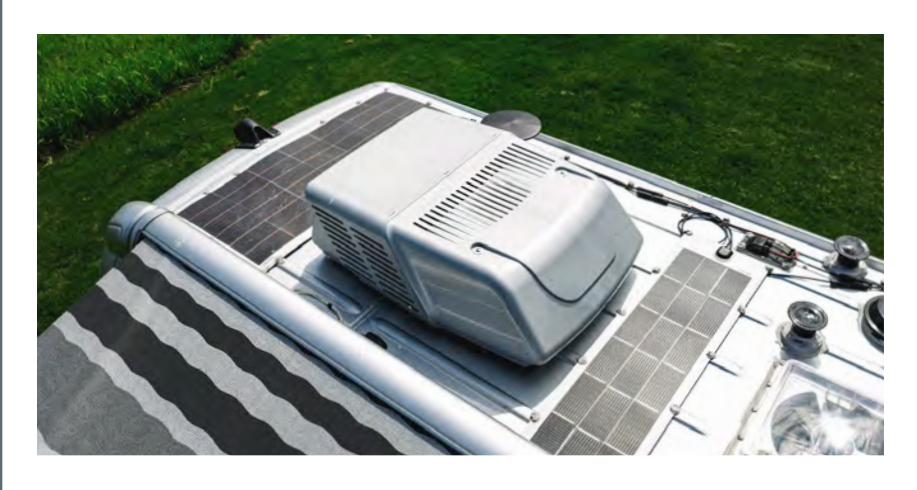
1 240 watts of solar panels on the roof harvest the free, abundant power of the sun.
