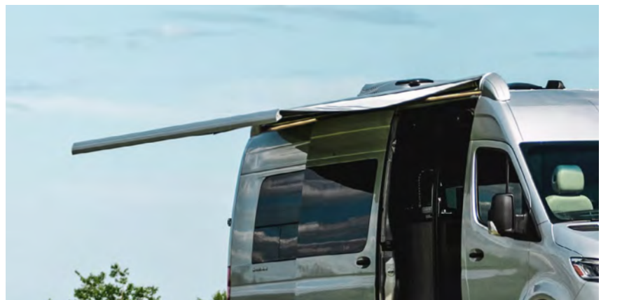
2 The powered awning extends and retracts at the push of a button.
