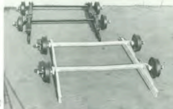
Dura-Torque axle (bottom) shows how torsion bars replace old fashioned leaf springs. Spring trouble is eliminated!
